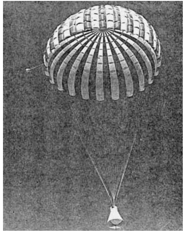
Figure 18. Main 63-foot ringsail parachute.
