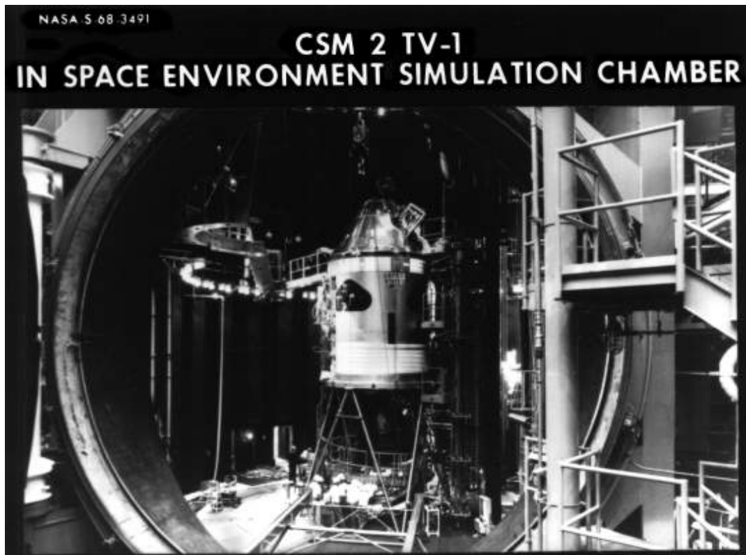
Command and service modules 2TV-1 in the space environment simulation chamber at Manned Spacecraft Center. Hinges for the huge door to close the chamber are at extreme left. Astronauts Kerwin, Brand, and Engle spent a week in this craft under operational space conditions in 1968.
