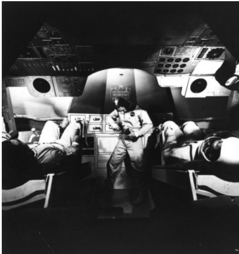
Interior of a partial full-scale mockup of the Apollo command module. In flight, the center couch would be removed as shown), giving better access to the instrument panel and lower equipment bay.
