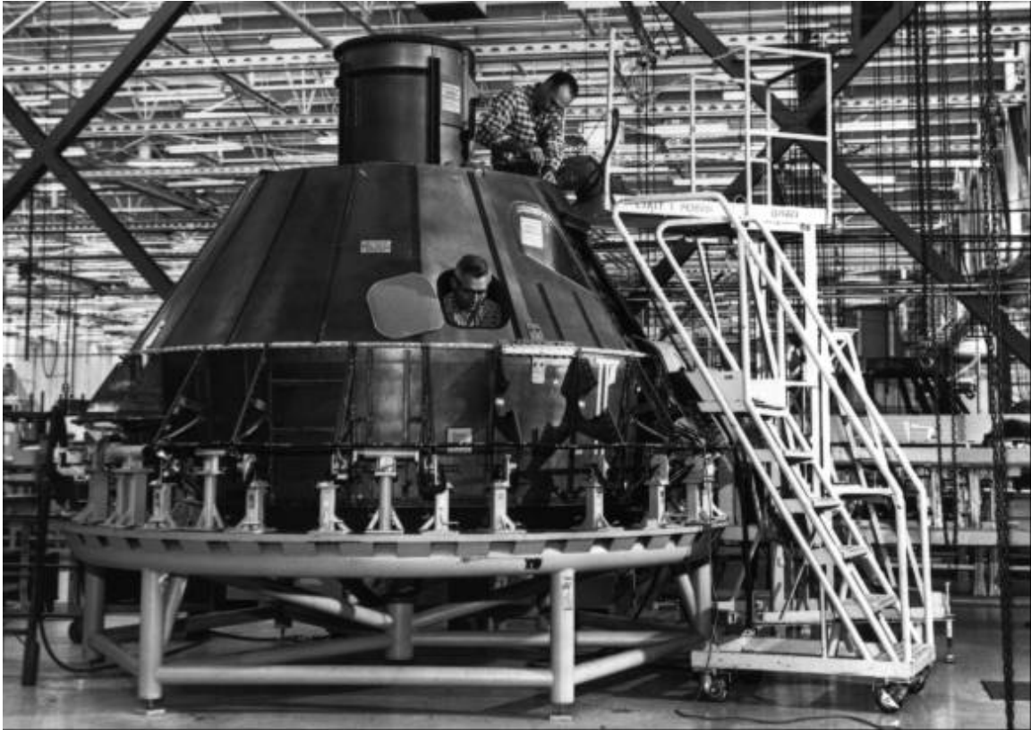
The cabin section (or primary structure) of the CM is assembled at North American in 1965.
