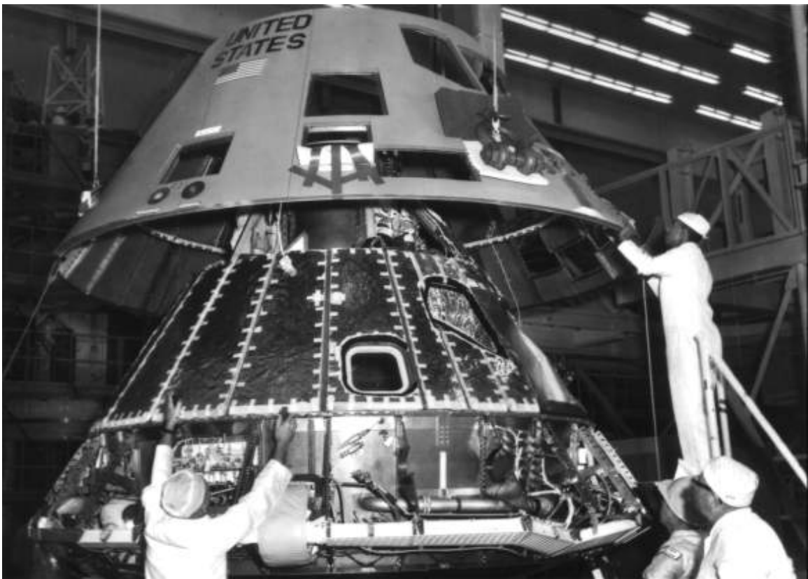
Technicians work on the central heatshield, the two men on the sides applying heat-protection ablative material with caulking guns.
