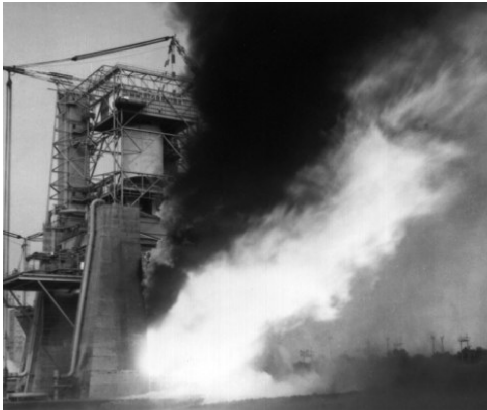
S-IC-T is fired for 2 1/2 minutes at Marshall in an August 1965 ground test.
