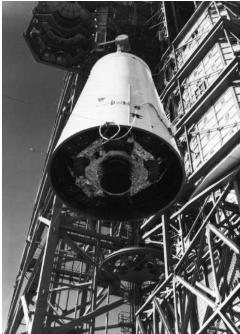
At right below, LM-1 inside the adapter is hoisted to the top of Saturn launch vehicle 204.
