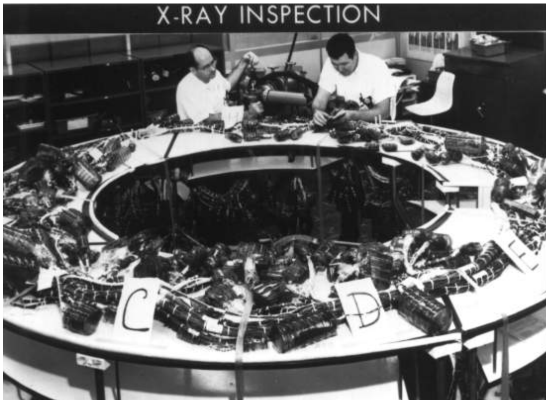
The CM wiring harness goes through x-ray inspection.
