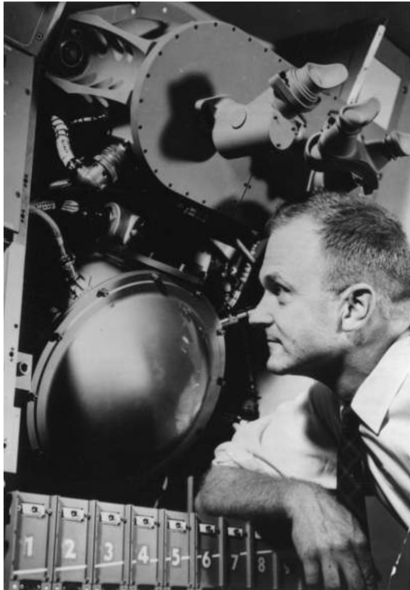
David G. Hoag, technical design director at the laboratory, examines the inertial measuring unit that would measure changes in Apollo spacecraft velocity when propulsion systems were fired.
