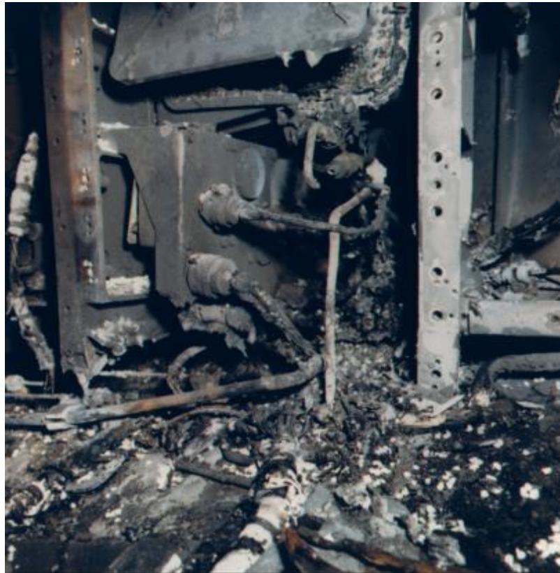
The environmental control system's instrumentation harness after the command module 012 fire that took the lives of Grissom, White, and Chaffee on 27 January 1967.
